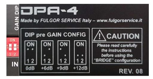
Refer to the table in order to determinie the desired input gain. Normally you work at 0dB, but t is possible to choose between 6-9-12 dB.
